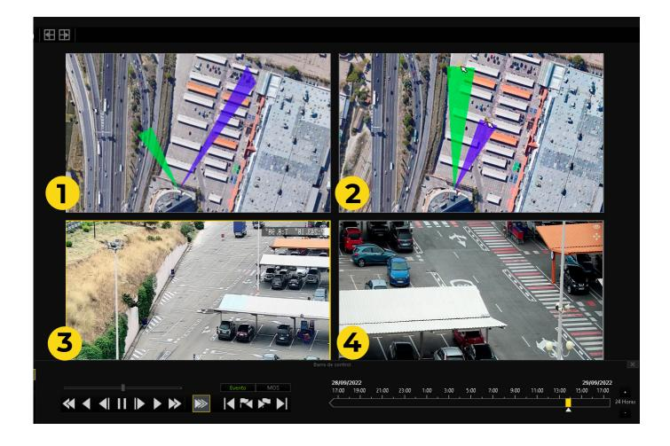
In the first image we can see the map and, represented in green and purple, the field of view of the cameras according to the selected focal length.
